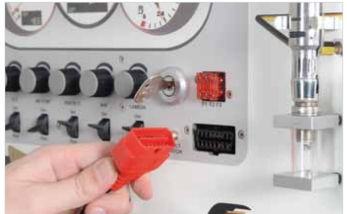
Using the OBD II terminal you can connect any OBD II-capable diagnostics tester and read out important data needed for trouble shooting.
